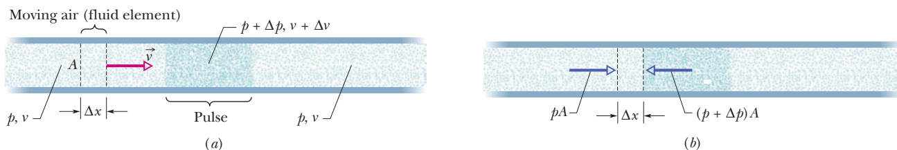
Figure 17-3 A compression pulse is sent from right to left down a long air-filled tube. The reference frame of the figure is chosen so that the pulse is at rest and the air moves from left to right. (a) An element of air of width \Delta x moves toward the pulse with speed v . (b) The leading face of the element enters the pulse. The forces acting on the leading and trailing faces (due to air pressure) are shown.
