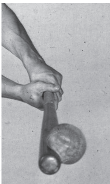
The collision of a ball with a bat collapses part of the ball.
